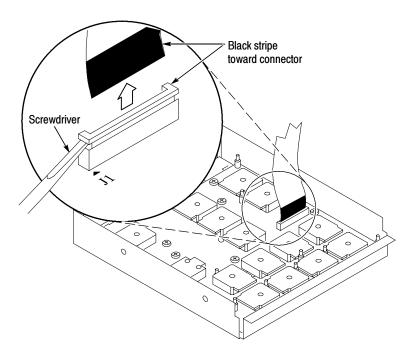
Figure 6-10: J1 flex cable connector removal
