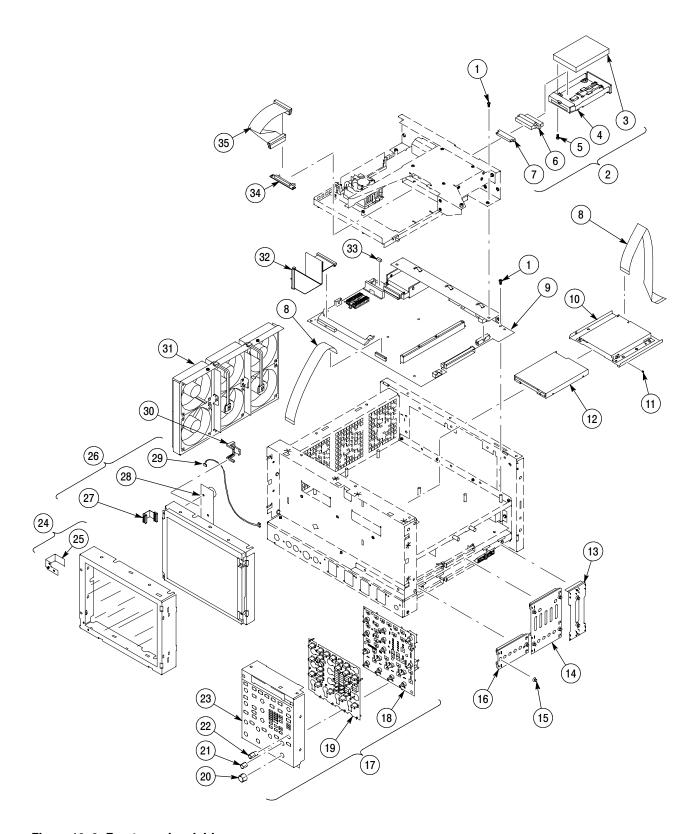
Figure 10-2: Front panel and drives
