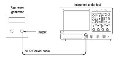
Figure 4-22: Initial test hookup
