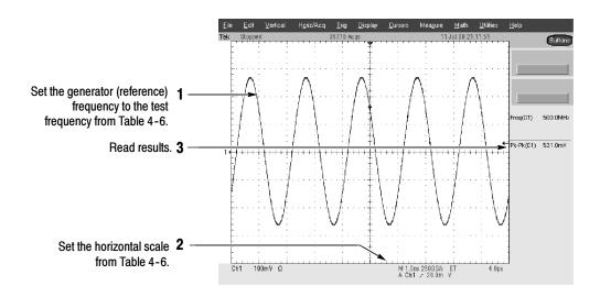
Figure 4-16: Measurement of analog bandwidth
