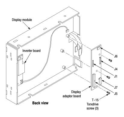
Figure 6-14: Display adaptor board removal
