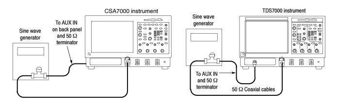
Figure 4-27: Initial test hookup
