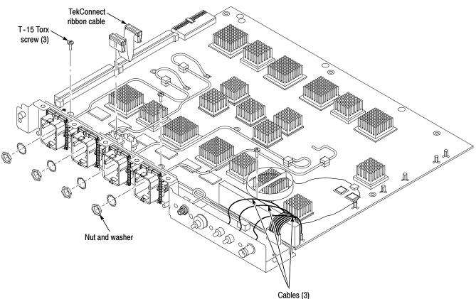
Figure 6-30: Front panel combination assembly removal
