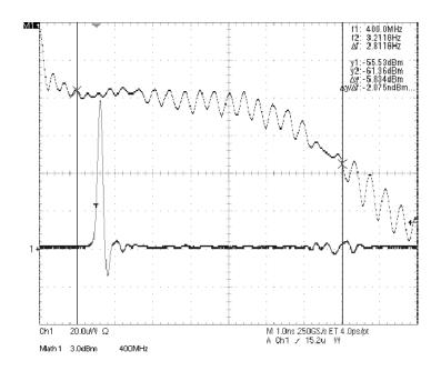
Figure 4-46: Optical impulse response
