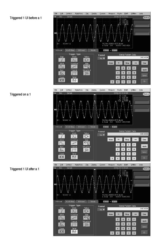
Figure 4-37: Isolated 1 triggering
