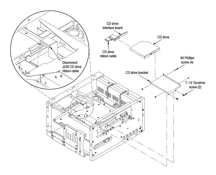
Figure 6-20: CD drive and bracket removal
