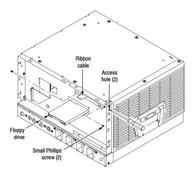
Figure 6-17: Floppy disk drive removal
