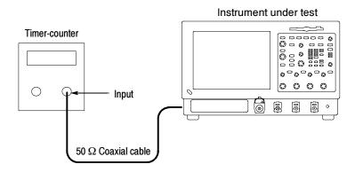
Figure 4-21: Initial test hookup
