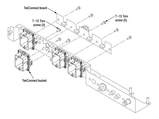
Figure 6-31: TekConnect board and TekConnect bucket removal
