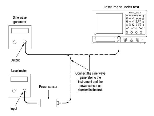
Figure 4-48: Equipment setup for maximum amplitude
