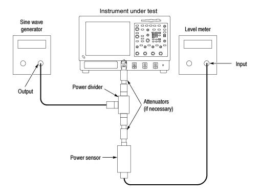
Figure 4-47: Sine wave generator leveling equipment setup
