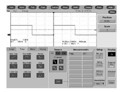
Figure 4-32: Measurement of probe compensator frequency
