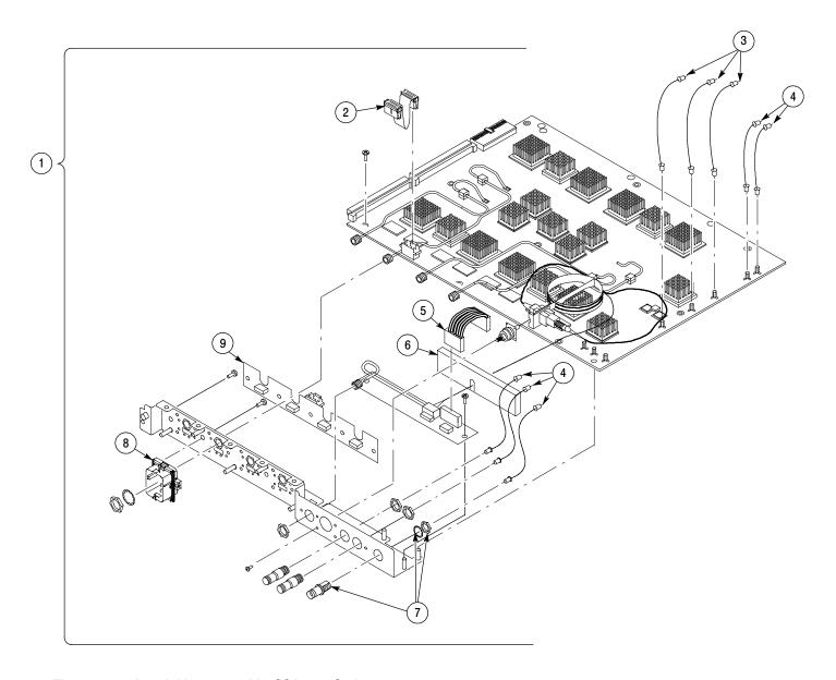
Figure 10-4: Acquisition assembly, CSA7000 Series
