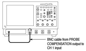
Figure 4-4: Setup for time base test
