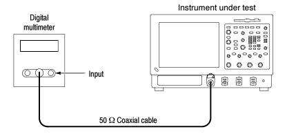
Figure 4-20: Initial test hookup
