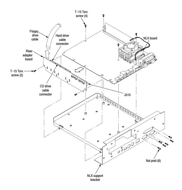
Figure 6-26: Riser adapter and NLX board removal
