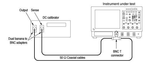
Figure 4-7: Initial test hookup
