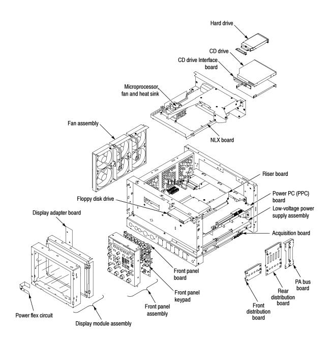
Figure 6-8: Internal modules
