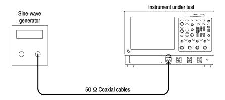
Figure 4-35: Initial test hookup
