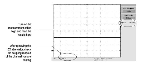
Figure 4-14: Check of maximum input voltage
