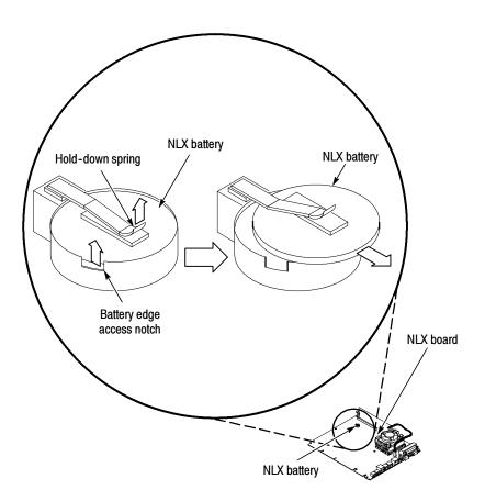
Figure 6-24: NLX battery removal
