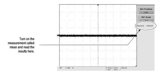
Figure 4-12: Measurement of offset accuracy
