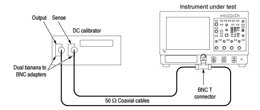
Figure 4-9: Initial test hookup
