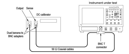
Figure 4-11: Initial test hookup
