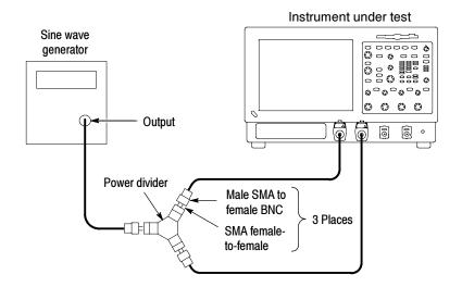
Figure 4-17: Initial test hookup
