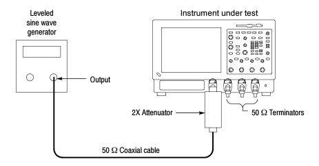
Figure 4-19: Initial test hookup
