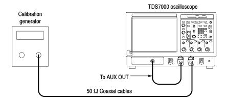
Figure 4-29: Initial test hookup
