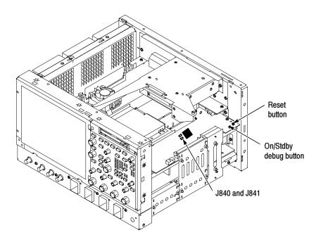
Figure 6-41: Location of jumpers and reset button
