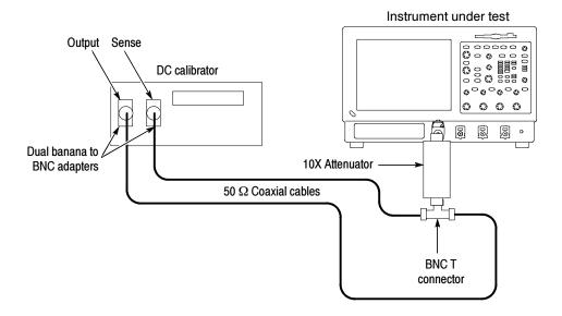
Figure 4-13: Initial test hookup
