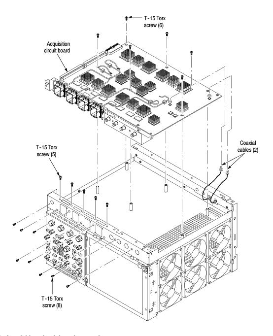
Figure 6-32: Acquisition circuit board removal
