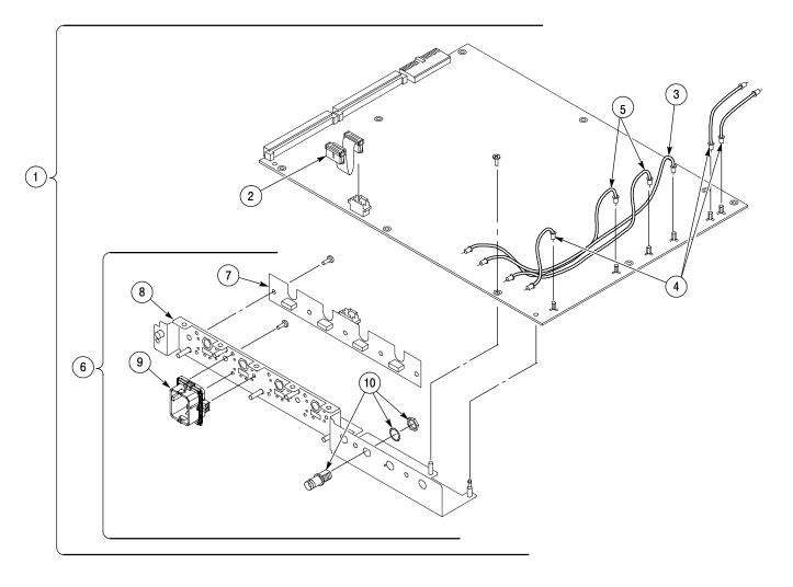
Figure 10-5: Acquisition assembly, TDS7000 Series
