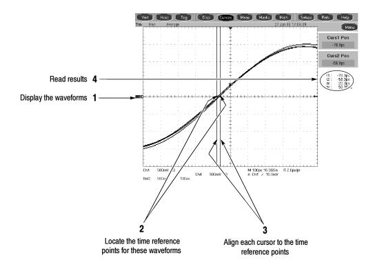
Figure 4-18: Measurement of channel delay
