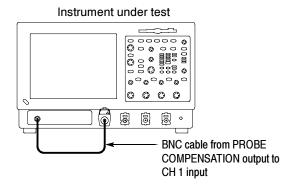
Figure 4-5: Setup for trigger test
