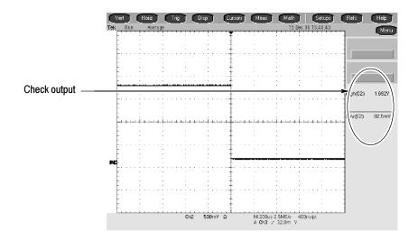
Figure 4-30: Measurement of trigger out limits
