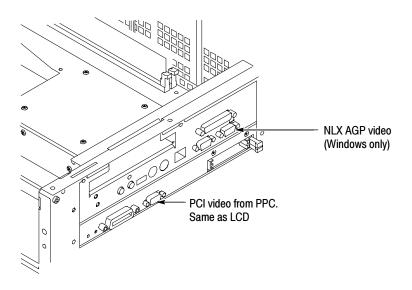
Figure 6-40: PCI and NLX video connectors
