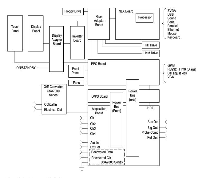
Figure 9-1: Instrument block diagram
