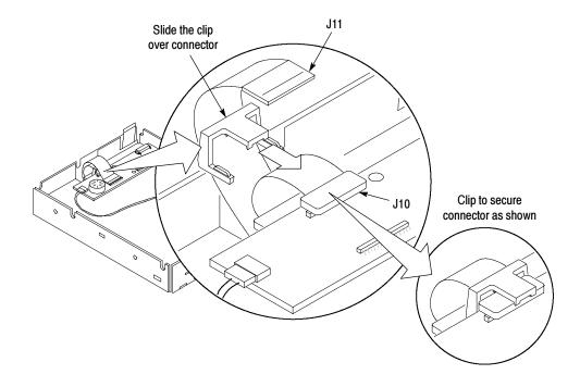
Figure 6-15: Cable clip removal
