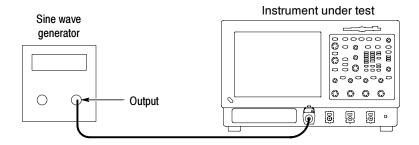
Figure 4-15: Initial test hookup
