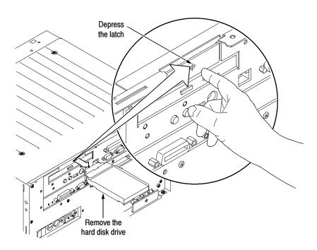
Figure 6-18: Hard disk drive removal
