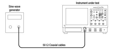
Figure 4-39: Initial test hookup
