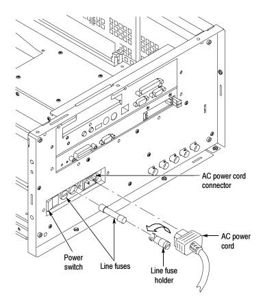
Figure 6-1: Line fuse and line cord removal
