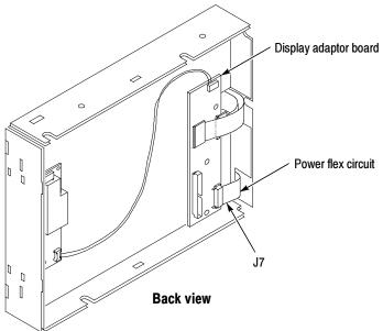
Figure 6-16: Power flex circuit removal
