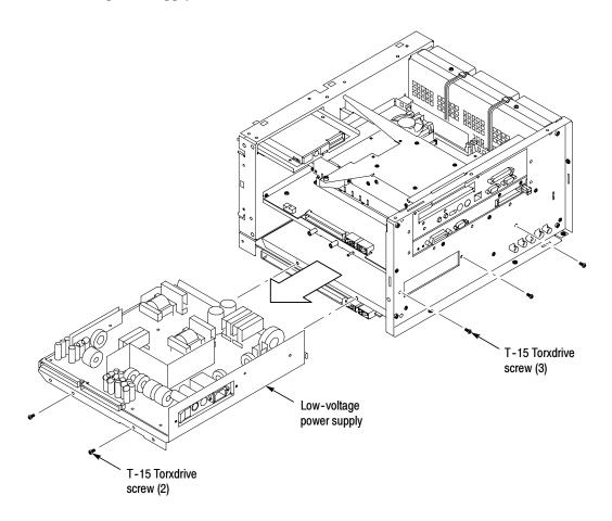
Figure 6-23: Low-voltage power supply removal
