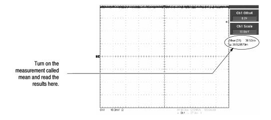
Figure 4-10: Measurement of DC gain accuracy
