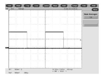
Figure 4-34: Measurement of probe compensator amplitude
