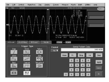
Figure 4-38: N modulo 3 triggering
