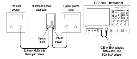
Figure 4-43: Initial test hookup
