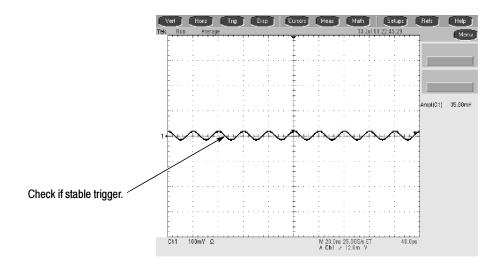
Figure 4-28: Measurement of trigger sensitivity - 50 MHz results shown
