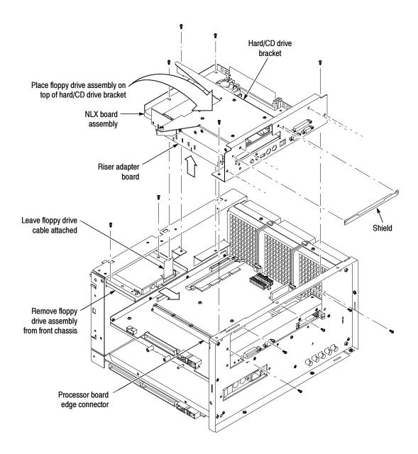
Figure 6-25: NLX assembly removal
