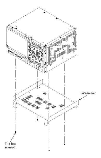
Figure 6-4: Bottom cover removal
