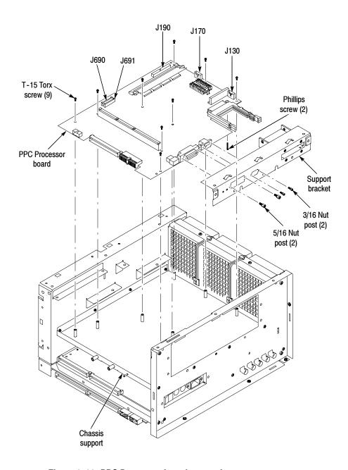
Figure 6-28: PPC Processor board removal
