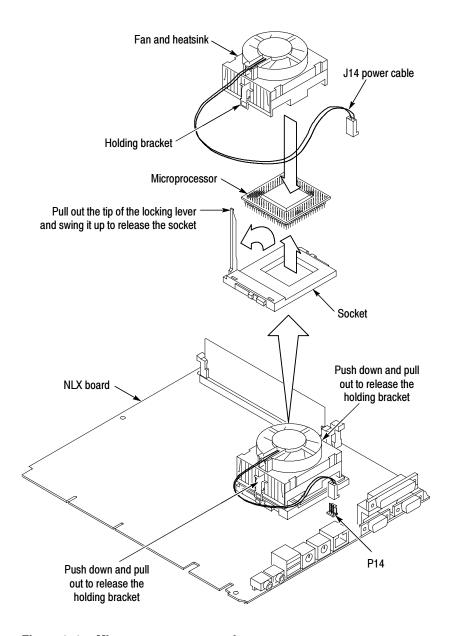
Figure 6-27: Microprocessor removal
