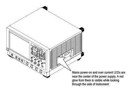
Figure 6-36: Location of power-on and over current LEDs
