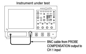
Figure 4-31: Initial test hookup
