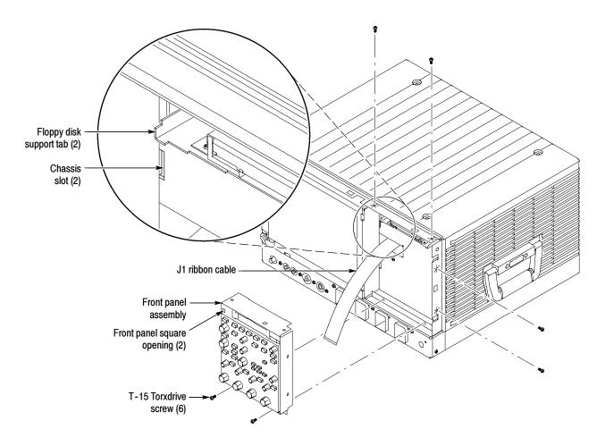
Figure 6-9: Front-panel assembly removal
