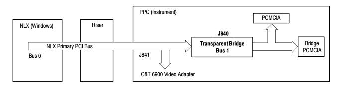
Figure 6-39: The three PCI busses
