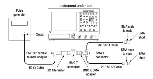
Figure 4-24: Delta time accuracy test hookup
