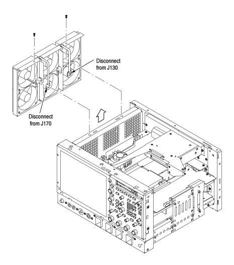
Figure 6-21: Fan assembly removal
