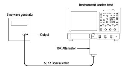
Figure 4-25: Initial test hookup
