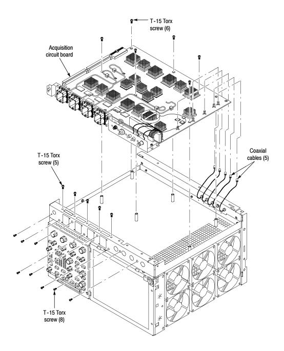
Figure 6-29: Acquisition circuit board removal
