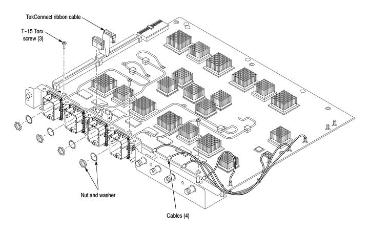
Figure 6-33: Front panel combination assembly removal
