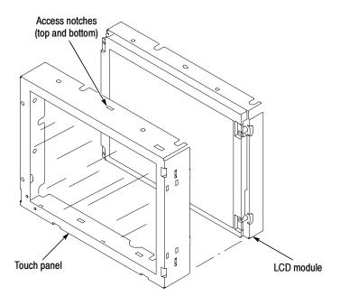
Figure 6-13: Touch panel and LCD assembly removal
